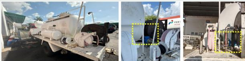
Gambar 39 Implementasi Instalasi Strainer Two Line
